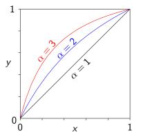
If the relative volatility between two components is equal to one, separation is not possible by distillation. The larger the value of  $\alpha$ , above 1.0, the greater the degree of separability, i.e. the easier the separation.
