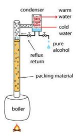
Without reflux, the possible separation is equal to that from a single-stage.
