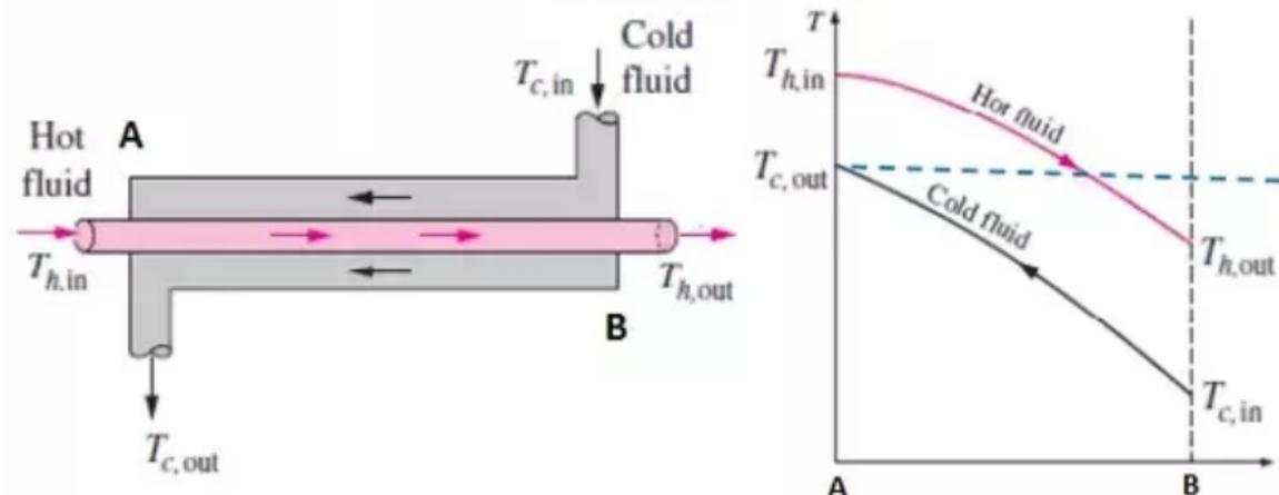
$T_{c,out}$ , out can exceed  $T_{h,out}$ .
