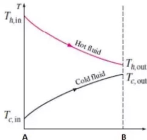
$T_{c,out}$ , cannot exceed  $T_{h,out}$ .
