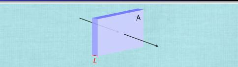
Consider the system shown above. The top, bottom, front and back of the cube are insulated, so that heat can be conducted through the cube only in the x direction. In this special case, heat flow is one dimensional. If sides were not insulated, heat flow could be two or three dimensional.
