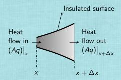
Let us consider a volume element of thickness  $\Delta x$  and having an area A normal to the coordinate axis x, as shown in the figure. The energy balance equation for this volume element is given by:
