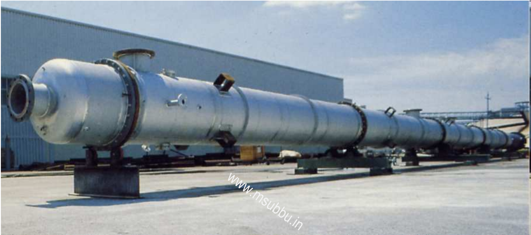
Distillation column D = 1400 \text{ mm} H=34000 \text{ mm}
