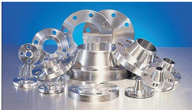
Specifications of standard flanges are given in ASME B16.5. The most common material is forged steel, with the specification of ASTM A181 or A105. The dimensions of flanges vary according to the pressure rating. The higher the pressure, higher will be the dimensions. The most common pressure ratings are: 150, 300, 600, 900, 1500, 2500 psig
