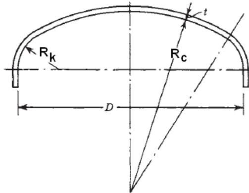
These heads have the crown radius equal to less than the diameter of the head. To reduce the stresses at the corner of the head, a knuckle is formed with a radius of at least 6% of inside diameter. The thickness of such heads is given by:
