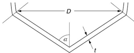
Thickness of conical heads with semi-apex angle  $\alpha$  is given by:
